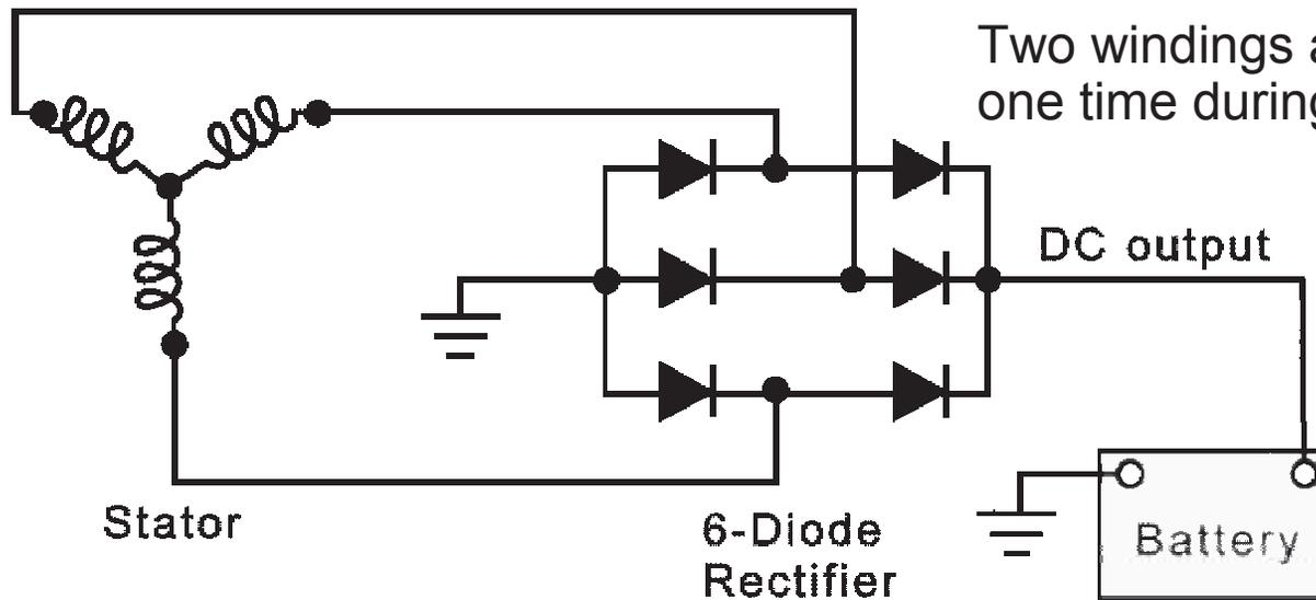
Two windings are in series at any one time during charge output.
