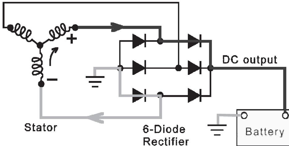
Now, in red B+ current passes through to the rectifier however, this time current has the opposite polarity. In green you can see the new return path.
