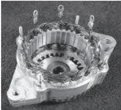
Wye wound stators have three windings with a common neutral junction. They can be identified because they have 4 stator lead ends.
