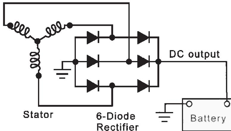
The Diode Rectifier Bridge is responsible for the conversion or rectification of the AC voltage into DC voltage.
