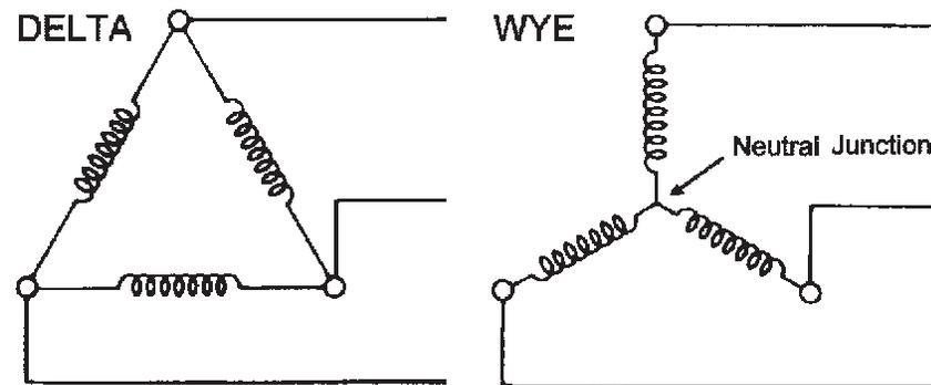
Wye style has four stator leads. One of the leads is called the Neutral Junction. The Neutral Junction is common to all the other leads.
