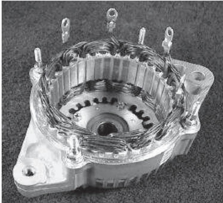
Two designs of stator winding are used. Delta and Wye.
