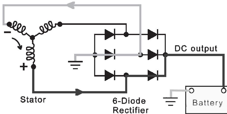
In red you can see B+ current pass through to the rectifier as it goes to the battery. In green you can see the return path.
