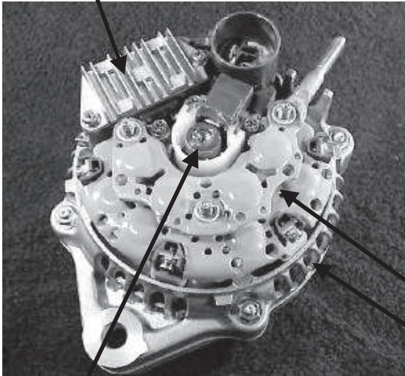
Slip Rings (part of the Rotor Assembly)
